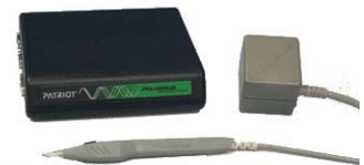
Digitizer stylus: a pen-like sensor that can track the position and angle of its tip
