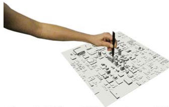
Small 16" x 16" version of the model was printed out by a Rapid Prototyping machine
