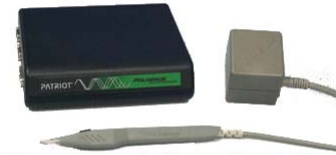
Digitizer stylus: a pen-like sensor that can track the position and angle of its tip
