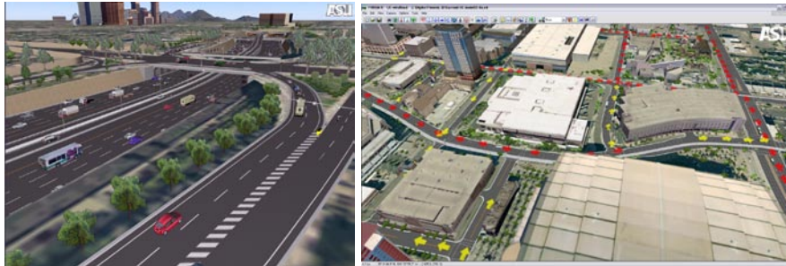
Figure3. Traffic moving along road network: using 3D automobile models (left) and with symbolic 3D arrows (right)
