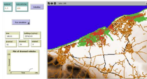
Figure 6. Screen shot image of agent-based model to simulate flood and traffic impacts
