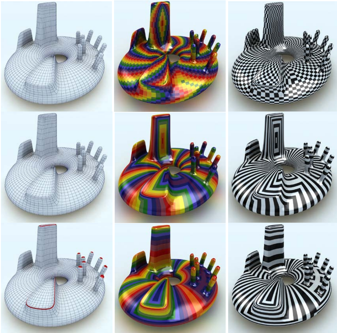
Figure 8. Samples of Generated Design Pattern: Original Mesh with Initial Selected Face(s) (left), the results of growing with colors (middle) and black and white (right)
